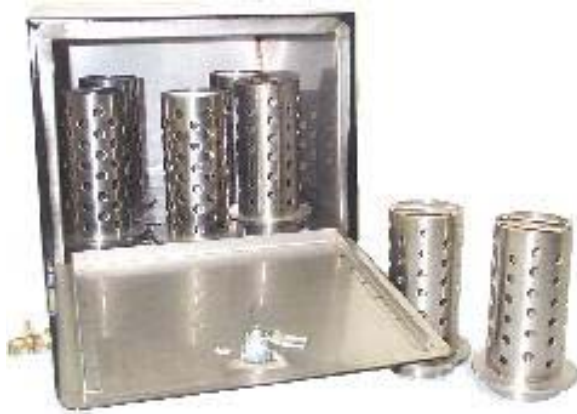
Steam dewaxers are available in different sizes. This one can hold several flasks. Photo courtesy of S. Sassounian.
